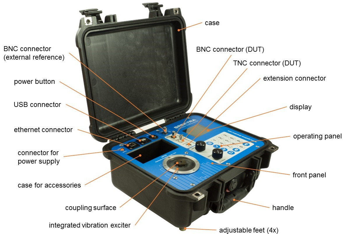
Figure 3-1: Components of the product (shown without power supply and accessories)
