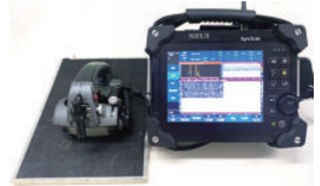
Honeycomb CFRP inspection
