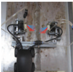
Dual-side Butt Weld Inspection
