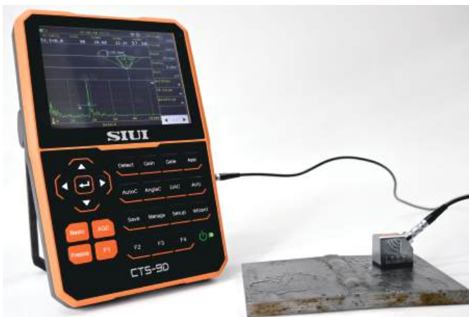
UT inspection for butt weld
