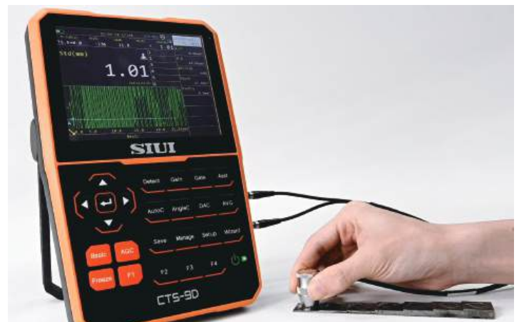
Thickness measurement on step-block
