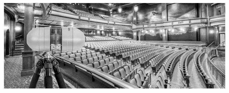
Qoms<sup>2</sup> is highly accurate at a maximum sound power level of 110 dB and shows an omnidirectional pattern over large frequency bands.
