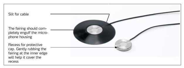
Fig. 5. Mounting the 40LA: Mounting the rubber fairing.
