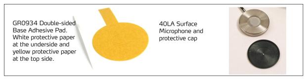
Fig. 3. Mounting the 40LA with double-sided adhesive pad for securing the fairing.
