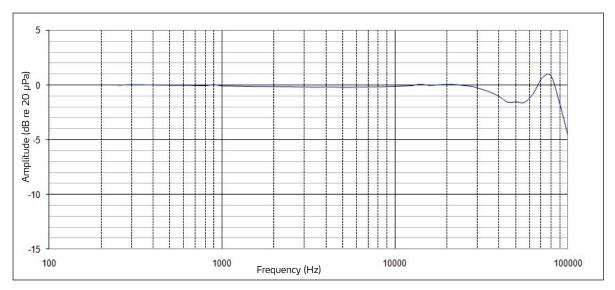
**Fig. 1.** Typical pressure frequency response of 40LA.
