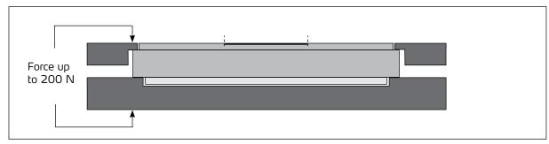
Fig. 10. Example of a mounting method where force is applied only to the upper housing.
