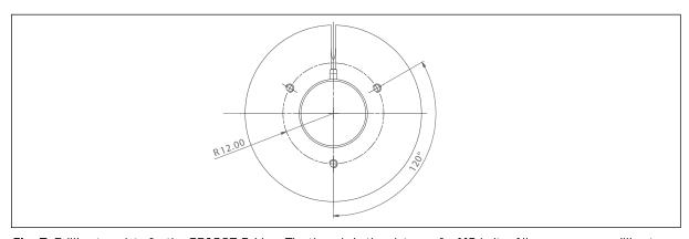
**Fig. 7.** Drilling template for the GR1297 Fairing. The threads in the plate are for M2 bolts. All measures are millimeters.
