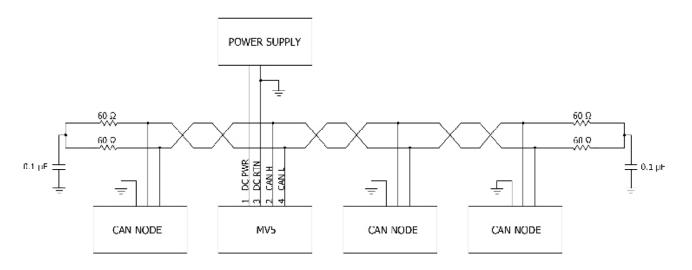
LORD recommends <u>split termination</u> on both ends of the cable for optimum EMC performance.
