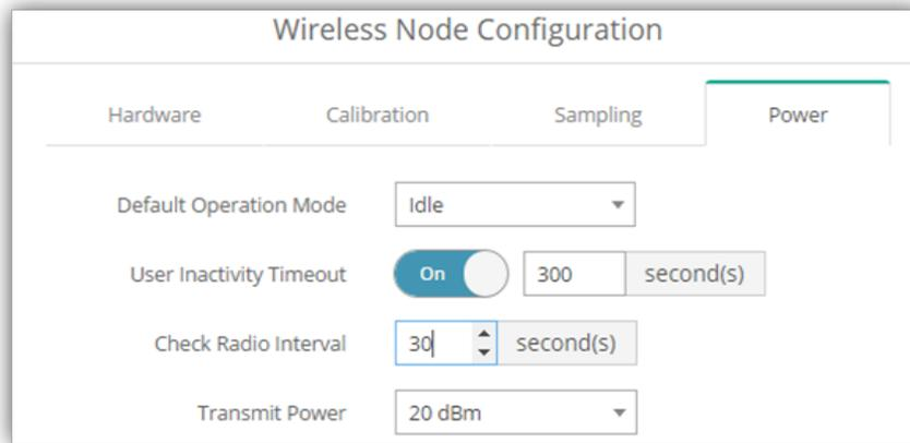
Figure 14. Node Configuration Power Menu
