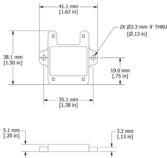
Figure 33. Installing the Mounting Board
