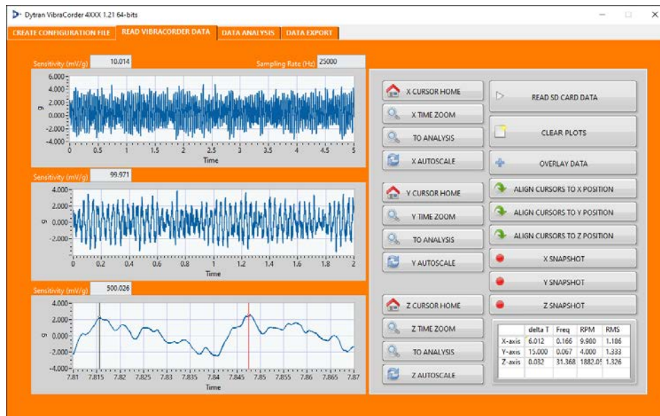
Figure 9: Channel three data of 1882 RPM (31.4 Hz) Engine Vibration at 1.326 g RMS.
