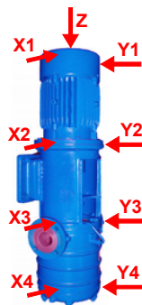
Figure 12: Measuring Points on Machines with Vertical Rotors
