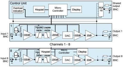
Figure 4: Block diagram
