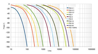
Figure 12: Phase response of M208B with different low pass filters FB2-...
