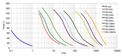
Figure 11: Phase response of M208B with different high pass filters FB3-...
