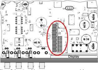
Figure 7: Location of the constant current source module
