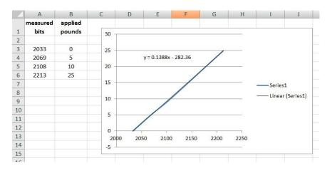
Figure 51 - Slope and Offset Values
