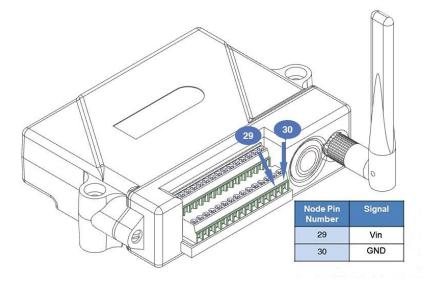
Figure 53 - External Power Connection
