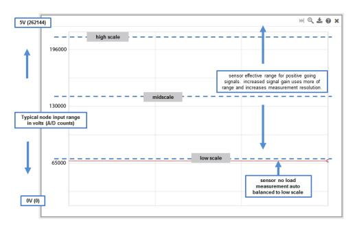
Figure 52 - Differential Input Resolution and Offset (18-bit Node)
