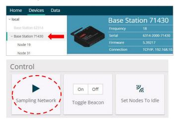
As a group, they will all be set to the same sampling mode. When the Base Station is selected, all the nodes will appear in a list with a check mark to the left, all of the nodes checked off will be included in the sampling. Uncheck the nodes to be excluded from the sampling.
