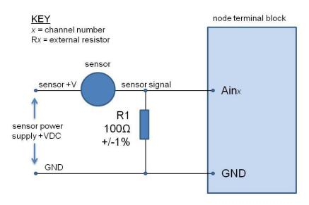
Figure 37 - Small Current Measurements
