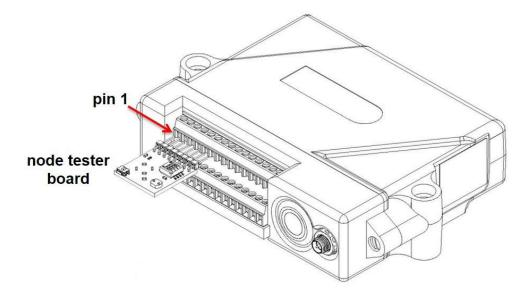
Figure 54 - Node Tester Board Installation
