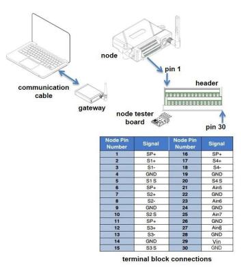
Figure 6 - System Connections
