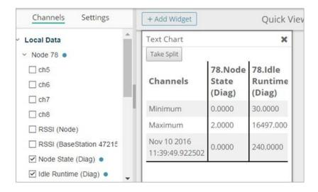
Figure 4 - Viewing Node Diagnostic Data
