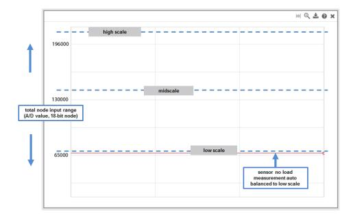
Figure 48 - Offset Scale Setting
