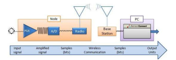
Figure 32 - Differential Channel Signal Processing
