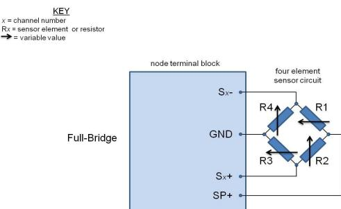
Figure 33 - Full Bridge Wiring
