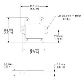
Figure 33. Installing the Mounting Board
