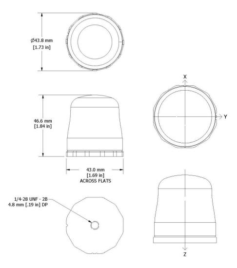
Figure 33 - Mounting the Node
