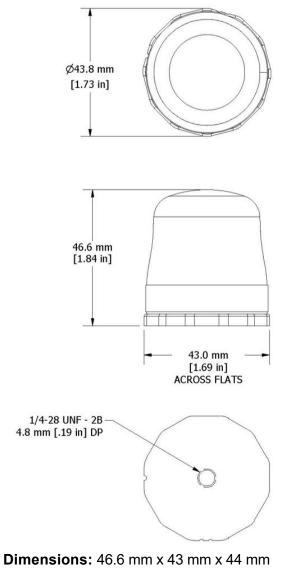
Mounting: ¼ - 28 UNF - 2B 4.8 mm [.19 in] DP. Weight: With 3batteries: 122 grams Enclosure Environmental Rating: IP67
