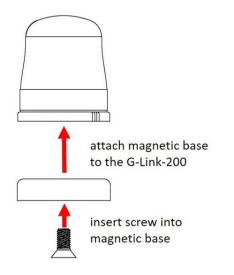
Figure 34 - Installing The Magnetic Base
