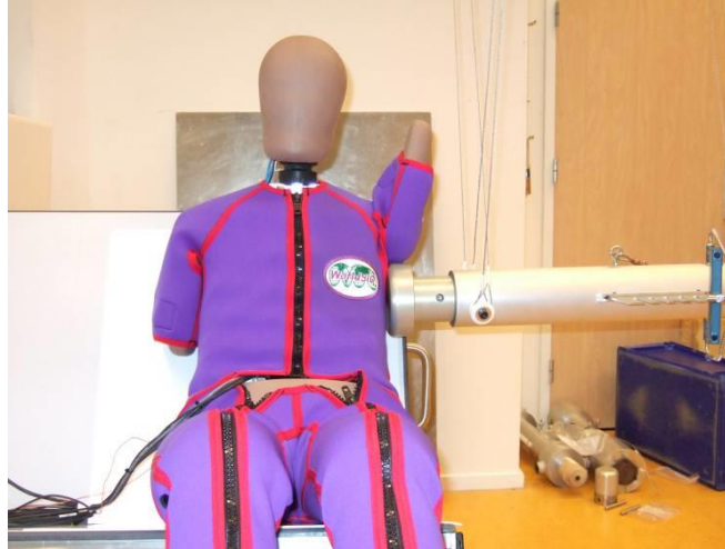
Figure 9.9 — Thorax test without arm, dummy and arm position
