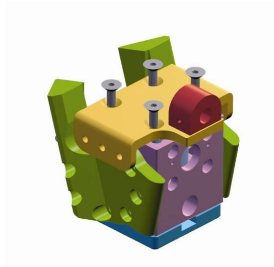
Figure 6.12 - Removing the lower lumbar mounting bracket weldment
