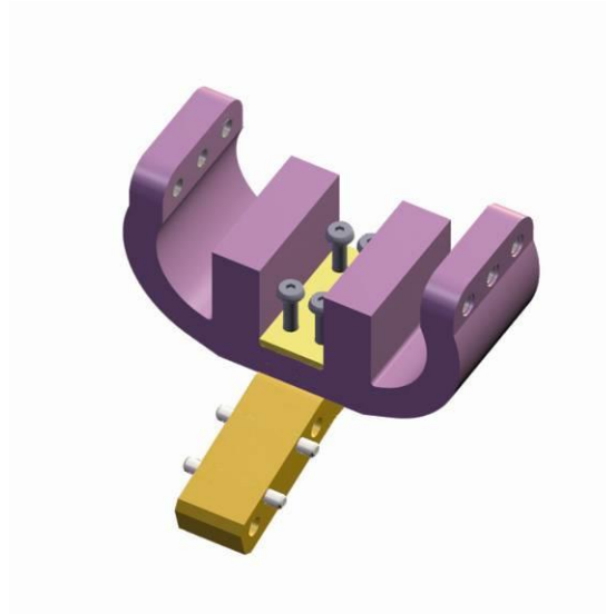
Figure 6.11 - Separating the upper lumbar clamping plate and lumbar mounting wedge
