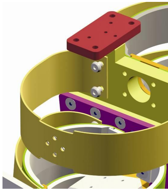
Figure 4.5 - Detaching the rib from the spine box at the rear
