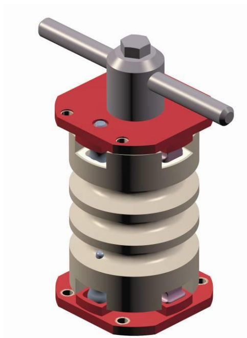
Figure 3.4 - Removing half-spherical screws and retaining plates
