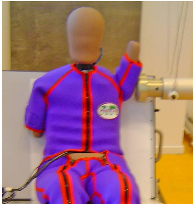
Figure 9.8 — Shoulder test, dummy and arm position
