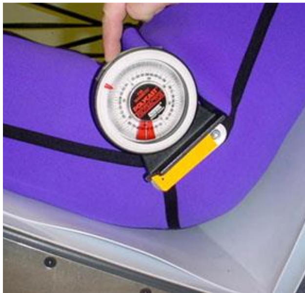
Figure 9.7 — Using an inclinometer with the H-point tool to check pelvis angle
