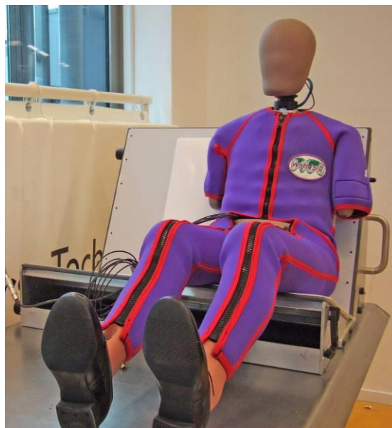
Figure 9.5 — Front view of setup for full dummy certification tests
