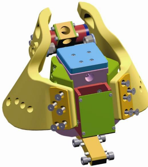
Figure 6.7 - Removing clamping plates to separate the pelvic bones
