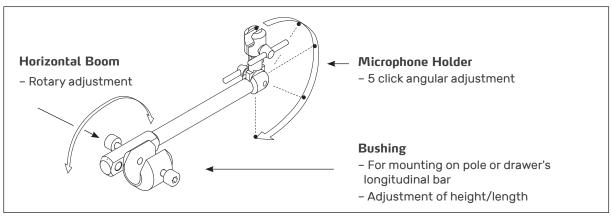
Fig. 3. The OPO041 Microphone Holder for attaching a microphone to the drawer.
