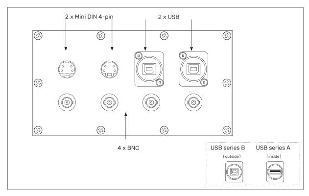
Fig. 6. The connector panel, outside view.
