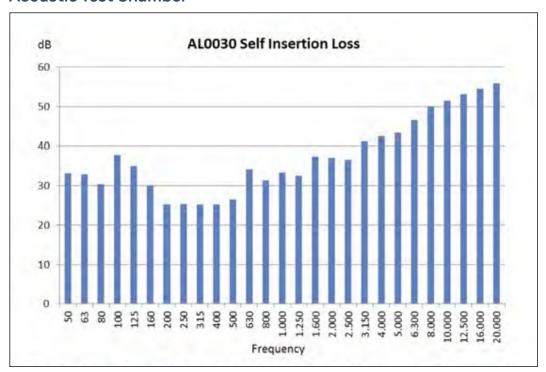
Fig. 7. SIL measured in reverberant conditions.
