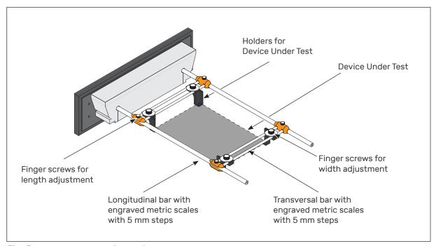
**Fig. 2.** The drawer and its fittings for holding the DUT. The drawer is shown without its telescopic mounting and sealing strip.
