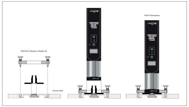
Fig. 2. How to mount and use the calibration adapter holder.
