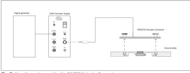
Fig. 3. Mounting and connecting the RA0310 Actuator Connector.
