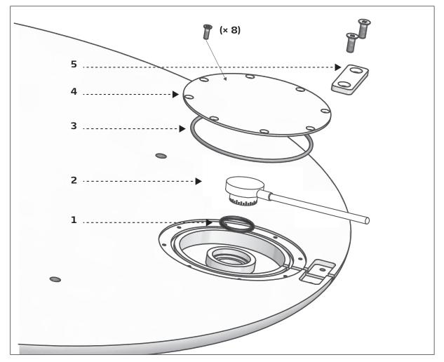
Fig. 1. A view of the order for assembling the parts of the 67AX/67AD.
