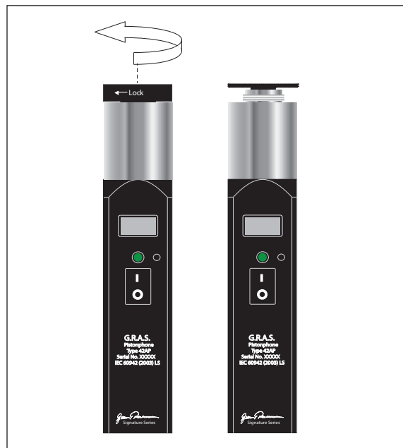
Fig. 13. Removing the collar before mounting the adapter
