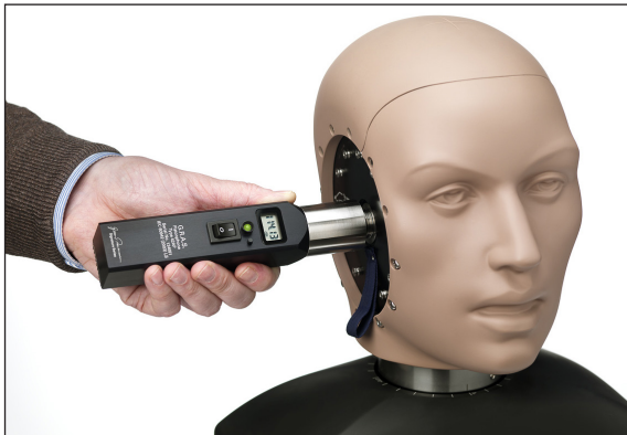
Fig. 19. Place the pistonphone onto the ear canal.
