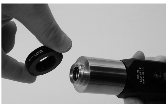
Fig. 17. Loosen the retention collar on the pistonphone.
