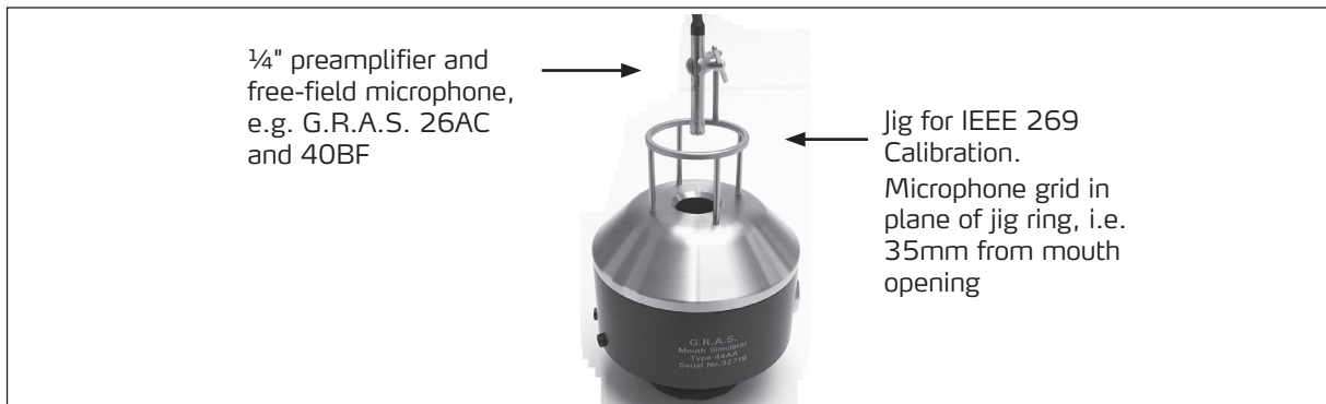
Fig. 9. Set up for calibrating the Mouth Simulator according to IEEE 269
