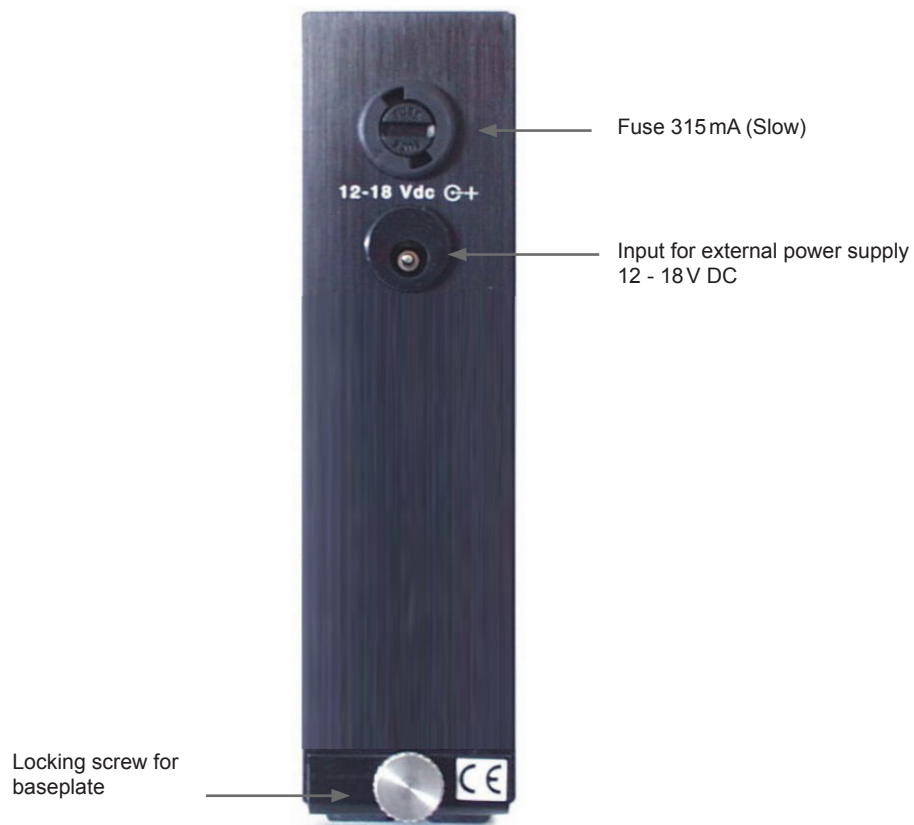
Fig. 2.4 Rear panel of the Intensity Power Module Type 12AB
