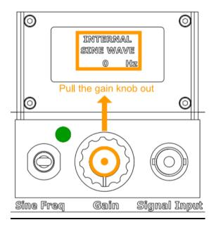
Raise or lower the Sine Frequency Generator Switch to the desired Sine frequency. Adjust the Gain of the amplifier by turning the Gain Knob clockwise. The frequency of the generated sine signal will be visible on the LCD Screen.
