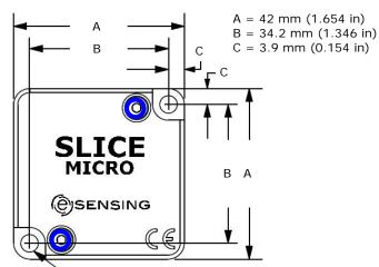
Ø4.3 mm (0.169 in) mounting thru holes x2 Accepts 6-32 (loose fit); M4 (free fit); 8-32 (tight fit)
