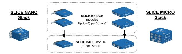
Example SLICE set-up with multiple Stacks:
