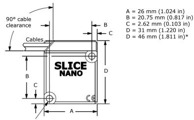
Ø3.2 mm (0.125 in) mounting thru holes x2 Accepts M2.5 (loose fit); 4-40 (free fit); M3 (tight fit)
