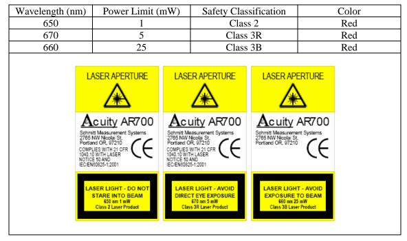
The laser safety classification reflects worst case situations. The laser is considered to be continuous, not pulsed. When the laser pulses in normal operation, the level of laser light does not increase.
