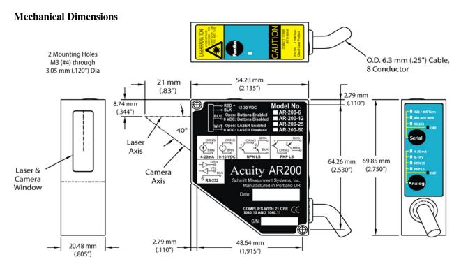
Figure 2 Mechanical Dimensions of AR200
