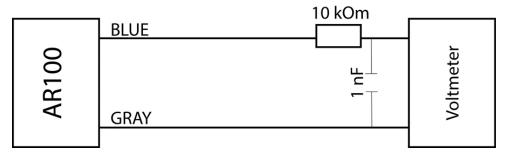
Figure 2 Wiring Diagram for Voltage output
