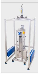
SE-201 pneumatic shock exciter to produce monopole shock pulse (half sine) as mechanical input signal for calibration purposes. Contains a digital laser interferometer (mach-zehnder) with positioning unit and damped tripod.
