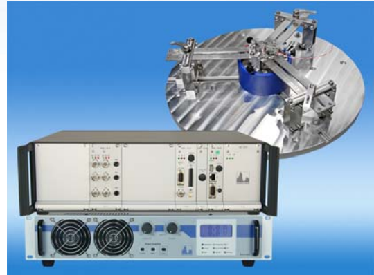
Vibration testing of sensors up to 400 g n using the VCS 201 on a vibration exciter SE-R101
