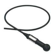
The D/70/H is a true spherical balanced element combined with a low noise differential pre-amplifier. Signals can be transmitted along cable lengths up to 500m, without any degradation. The preamplifier gain options of 20, 30 and 40 dB (are pre-set during manufacture) to suit the customer requirements.
