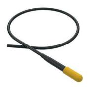
The D/300 miniature high frequency hydrophone is a versatile acoustic sensor, the spherical ceramic element retains an excellent spherical beam pattern up to 350 kHz. The robust construction of the D/300 enables it to operate at depths down to 700 metres.
