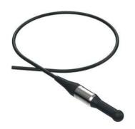
The D/140/H is a true spherical balanced element combined with a low noise differential pre-amplifier. Signals can be transmitted along cable lengths up to 250m, without any degradation. The preamplifier gain options of 20, 30 and 40 dB (pre-set during manufacture) are to suit customer requirements.
