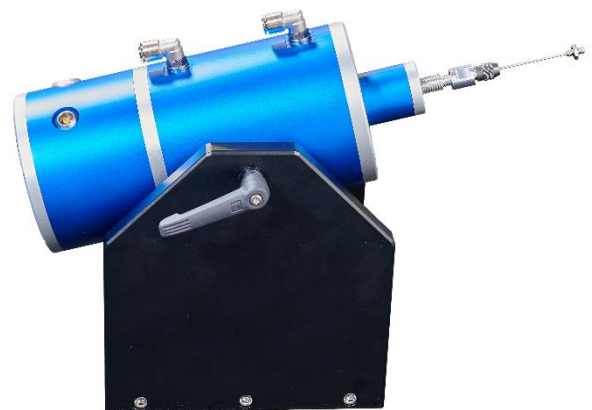
Figure 2: X-Act 325 shaker with collet and stinger for modal testing
