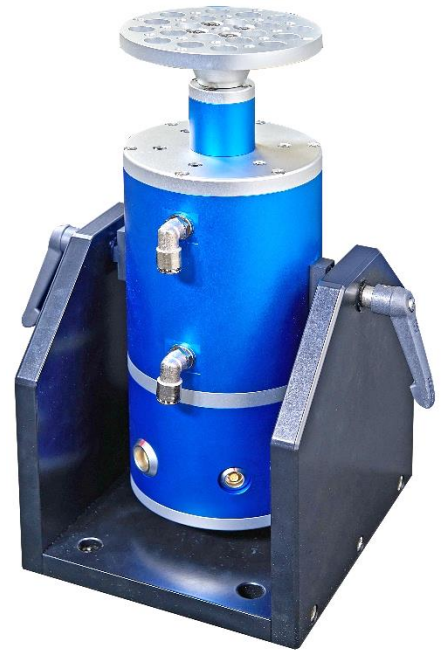
Figure 1: X-Act 325 shaker with 115mm mounting table for component testing
