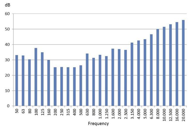
Self Insertion Loss measured in reverberant conditions
