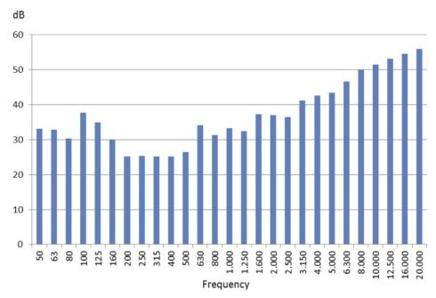
Self Insertion Loss measured in reverberant conditions
