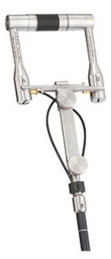
Freq range: IEC 61043 Class 1 Dyn range: 27 dB(A) to 146 dB Sensitivity: 12.5 mV/Pa Type 50GI-P is a sound intensity probe for direct connection to signal analyzers or data acquisition devices with IEPE inputs. The probe includes a pair of phasematched prepolarized precision microphones which meet the requirements in IEC standard 61043 for a class-1 intensity probe.
