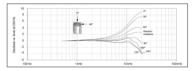
Free-field corrections for different angles of incidence
