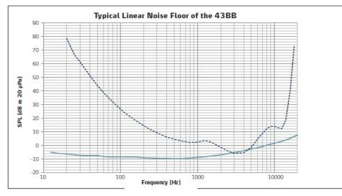
The noise floor (solid line) is typically below the threshold of human hearing (dashed line).
