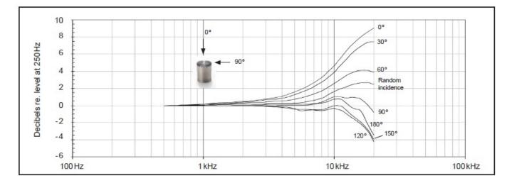
Free-field corrections for different angles of incidence
