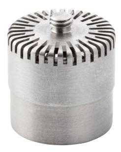
Freq response: IEC 61043 Dyn range: 20 dB(A) to 157 dB Sensitivity: 25 mV/Pa The 40Al is an IEC 61094-compliant, WS2F ½" externally polarized sound-intensity microphone pair especially suited for sound-intensity and sound-power measurements, sound-source location and IEC 61043 Standard Instrumentation. Its equivalent prepolarized version is <u>GRAS 40GI</u>
