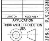
UNLESS OTHERWISE SPECIFIED INTERPRET DIM & TOL PER ASME Y14.5M - 1994. REMOVE BURRS. COUNTERSINK INTERNAL THDS 90° TO MAJOR DIA. CHAM EXT THDS 45° TO MINOR DIA. THD LENGTHS AND DEPTHS ARE FOR MIN FULL THDS: THDS PER MIL-S-7742. DIMENSIONS APPLY AFTER FINISHING.
