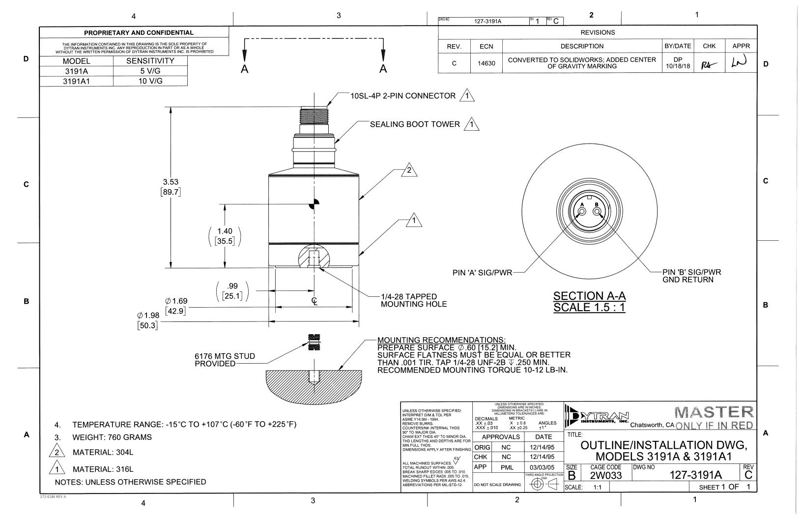
Model Number DOC NO PERFORMANCE SPECIFICATIONS PS3191A 3191A IEPE SINGLE AXIS ACCELEROMETER REV C, ECN 10367, 09/11/13
