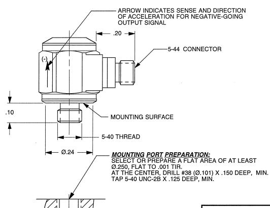
MASTER INSTRUMENTS, INC. ONLY IF IN RED CHATSWORTH, CA. 4X 6/10/04 Α PART NO. MODEL 3035C 11/15/99 DRAWN HECKED MAT'L N.C. R.A. NEXT ASSEMBLY USED ON DWG NO. **OUTLINE/INSTALLATION DRAWING,**
