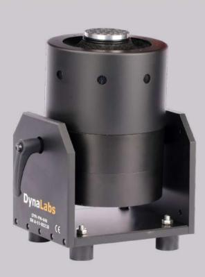
Permanent magnet shakers create motion by a pair of magnets and coils pushing and pulling each other. In fact, the technology inside is not different from that in loudspeakers and they are also called voice coils.
