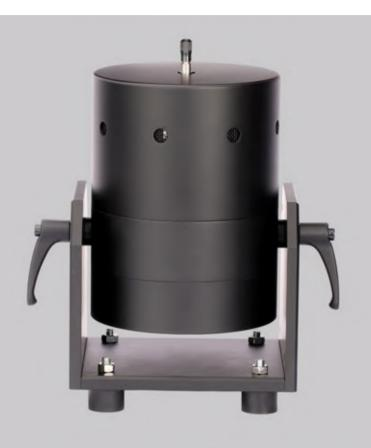
Both modal shakers and impulse hammers can be used in modal testing to excite the structures, but modal shakers have some advantages against impulse hammers such as cleaner and more accurate measurement data, the ability to test inaccessible points, and the capability to distinguish highly coupled modes. Modal shaker testing is also preferred for less noisy and more accurate results in many industrial applications.
