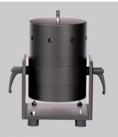
Both modal shakers and impulse hammers can be used in modal testing to excite the structures, but modal shakers have some advantages against impulse hammers such as cleaner and more accurate measurement data, the ability to test inaccessible points, and the capability to distinguish highly coupled modes. Modal shaker testing is also preferred for less noisy and more accurate results in many industrial applications.
