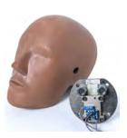
The A64C mounts on standard triaxial accelerometer mounting blocks and locations. Also works with all SLICE6 in-dummy DAS solutions!
