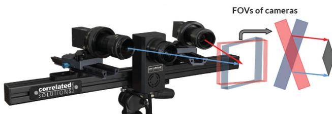
Effective usable FOV width is far smaller than for a single camera. Further depth-of-field for enhanced FOV requires a closed aperture, which reduces optical resolution due to the diffraction limit.
