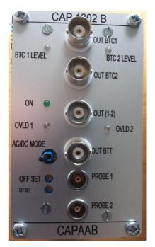
**Distance range**: From  $0 \rightarrow 2$  mm to  $0 \rightarrow 10$  mm according to the diameter of the double electrode® sensor used [pseudo triaxial type]
