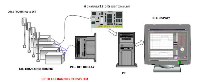
The **BTC** output of the CAP1802 conditioners are sent to **BTC acquisition** and processing system
