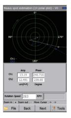
Find out the heavy spot location from a single coast-down measurement of couple balancing. 1X vibration.
