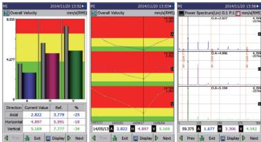
Triaxial measurement gives global view of machine conditions and saves work hours.
