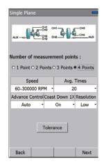
Select up to 4 measurement points for single or dual plane balancing.
