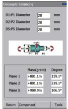
Conversion of dual plane balancing into static and
