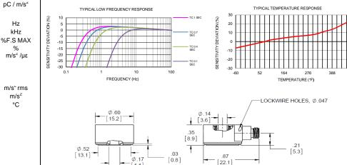
Units on the line drawing are in inches, units in brackets are in millimeters. Refer to 127-3221C for more information.
