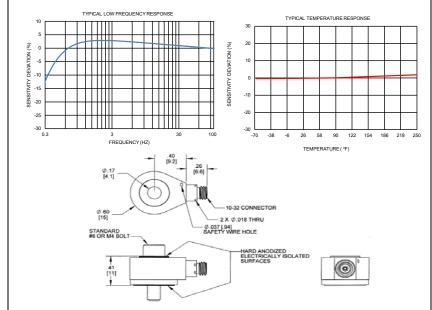
Units on the line drawing are in inches, units in brackets are in millimeters. Refer to 127-3211A for more information.
